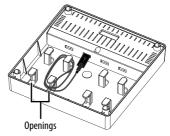
**4** Place the cover on the base so that the wire holes on the base and cover are aligned. Your cables should exit the base through the holes. Insert the dividers into the slots, as needed.
